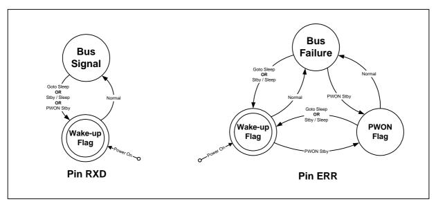
Figure 5 : State Diagrams, pins RXD and ERR
