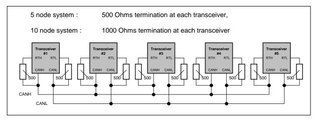
Figure 6 : Example Network with 5 nodes, 500 Ohms termination at each node
